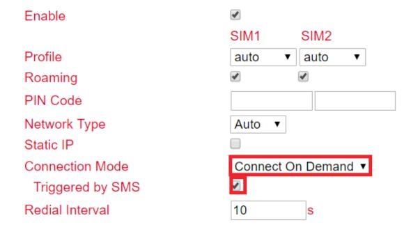
3) Under Connection Mode, select Connect on Demand and activate the field Triggered by SMS.
