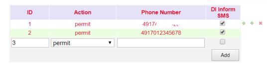
Tips:After enabled DI Inform SMS, router will send SMS when DI status changed.
